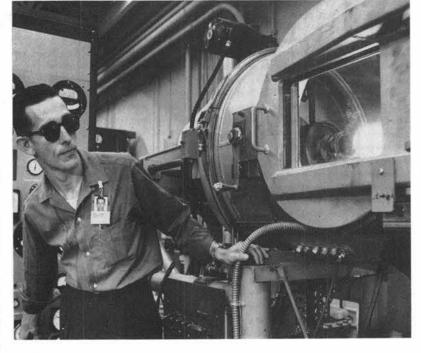
CONTROLS of 120-kw plasma generator are adjusted by James V. Williams (7131-1). Nozzle of plasma generator is visible through window.
